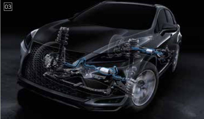
02 / Performance dampers The front and rear performance dampers enhance rigidity and vibration damping performance, to realize exceptional handling stability at the heart of sports driving enjoyment.
