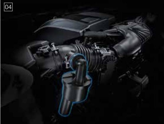
04 / Sound generator Heightening the emotion and excitement of sports driving, the sound generator boosts the sound pressure level in the engine air intake at different resonate frequencies, to generate a thrilling F SPORT engine note when you accelerate.
