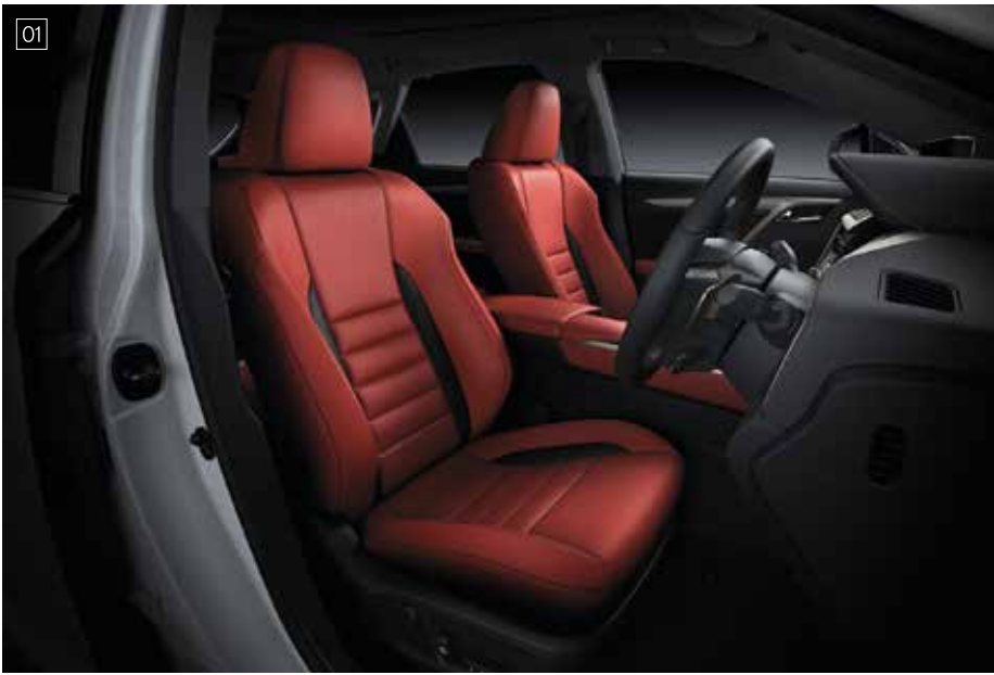
01 / F SPORT front seats The front sports seats are the product of an innovative 'integrated foaming' manufacturing process. They provide a blend of refined comfort with firm support and excellent holding performance for sports driving.
