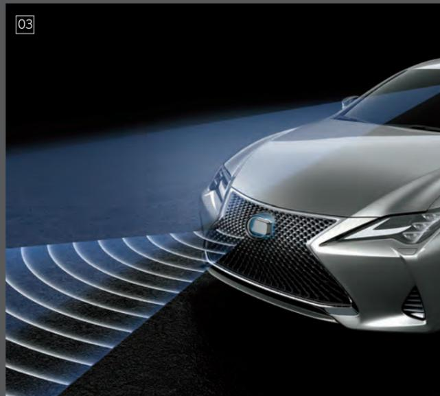
03 / Pre-crash Safety System When the radar and camera sensors detect a collision with a pedestrian, vehicle or obstacle ahead is likely, it alerts the driver and activates pre-crash brake assist when the driver depresses the brake pedal. If it determines a collision is difficult to avoid, the pre-crash brake and pre-crash seatbelts also operate. The dynamic radar cruise control uses the same radar and camera sensors to maintain your pre-selected distance behind the vehicle ahead.
