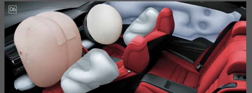
06 / SRS airbags To help reduce the impact to occupants in a collision, the RC is equipped with eight SRS airbags; dual-stage SRS airbags, SRS knee airbags and SRS side airbags for the front seats, and SRS curtain shield airbags for the door windows.\*
