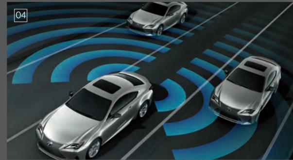
04 / Blind Spot Monitor System When the quasi-millimeter-wave radars in the rear bumper detect vehicles in adjacent lanes that aren't visible in the door mirrors, the system activates a warning indicator in the relevant door mirror the moment a vehicle enters this blind spot.
