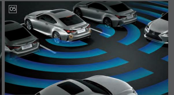
05 / RCTA (Rear Cross Traffic Alert) To assist safe reversing, RCTA uses quasi-millimeter-wave radars in the rear bumper to detect approaching vehicles in difficult-to-see areas behind the vehicle. When an approaching vehicle is detected, RCTA alerts the driver using a buzzer and indicator in the relevant door mirror.
