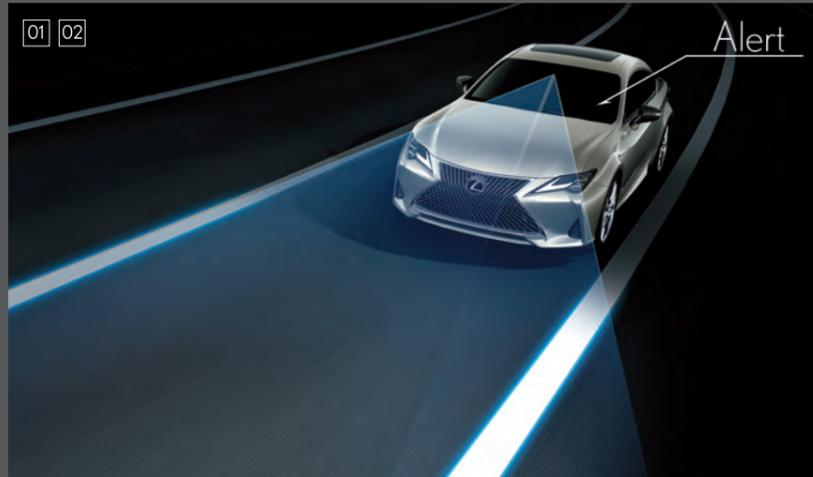
01 / LKA (Lane Keeping Assist) LKA alerts the driver with a buzzer and on the multi-information display if the system judges the vehicle is about to cross the lane markings without using the turn signals.\*
