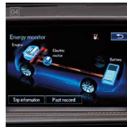
04 / Regenerative braking The regenerative brake system activates the motor as a generator while decelerating and braking, converting the moving vehicle's kinetic energy into electric energy and using it to charge the battery.
