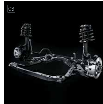
03 / Front suspension The MacPherson strut front suspension contributes to the excellent ride comfort and handling stability. The coil springs, stabilizers and shock absorbers were optimized to help realize excellent straight-line stability, for confident driving on various terrains.
