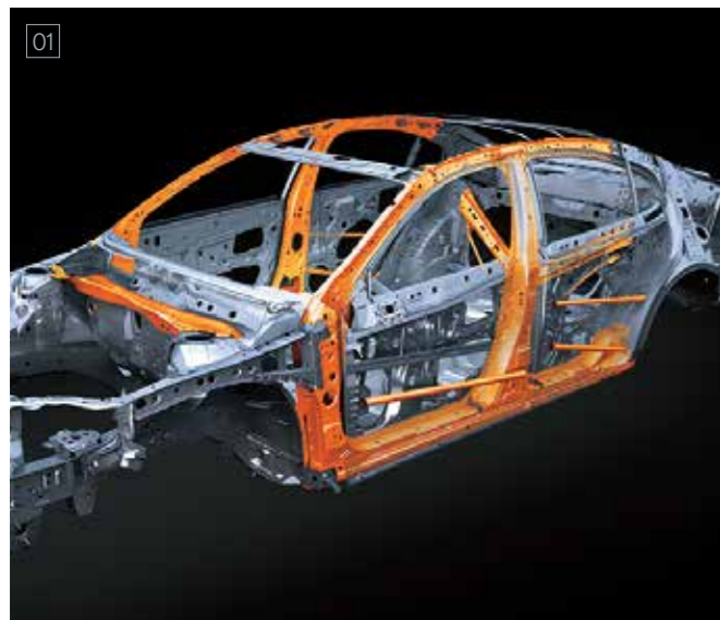
01 / Chassis The highly-rigid body structure of the ES enhances the basics of dynamic performance, including excellent straight-line stability, agile lane changing and ride comfort. Extensive use of high-tensile steel helps to optimize strength while keeping weight to a minimum. The high integrity cabin with front and rear crumple zones also contributes to occupant protection.
