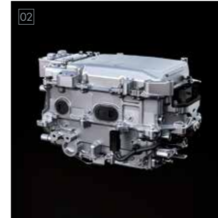
02 / Power control unit The brain of the Lexus Hybrid Drive-the power control unit optimizes control of DC electricity from the battery and AC electricity for driving the motor and generator. It also boosts battery voltage for extracting maximum power from the motor and generator.
