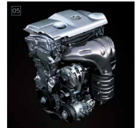
05 / 2.5-liter 4-cylinder Engine Compact and lightweight, the ES 250's engine realizes high performance, superb fuel efficiency, low emissions and outstanding quietness. Advanced technologies such as Acoustic Control Induction System (ACIS) and Dual VVT-i enhance torque and fuel economy across the entire driving range.
