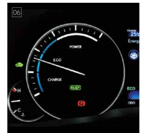
06 / Electric Vehicle (EV) Drive Mode EV-Drive Mode limits starting of the engine to enable the car to be driven using only motor power up to speeds of approximately 40km/h. It is designed to enhance quietness while driving in residential areas late at night and to reduce emissions in indoor car parks and garages.*
