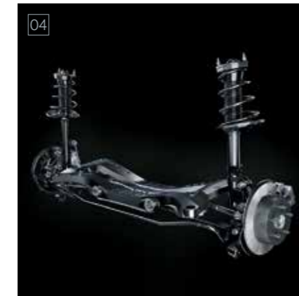
04 / Rear suspension The excellent handling stability and ride comfort are the product of optimizing the geometry and layout of the dual-link strut rear suspension. Close attention paid to reducing the weight of each component further contributes to both handling stability and excellent fuel efficiency.
