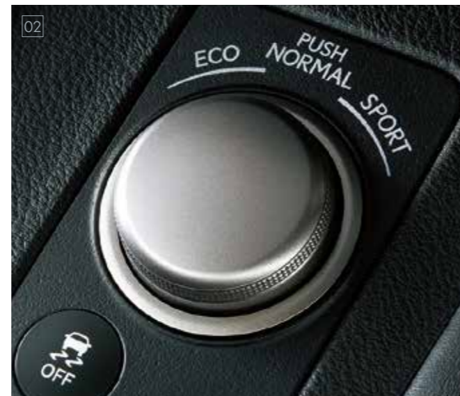
02 / Drive Mode Selector You can tune the performance of the ES to suit your driving mood. Selecting Eco Mode changes the throttle control and air conditioning characteristics, helping to reduce emissions and fuel consumption. Sport Mode adjusts the throttle control and Electric Power Steering (EPS) to give a more responsive and direct driving feel. Normal Mode optimally balances Eco Mode and Sport Mode attributes for everyday driving.
