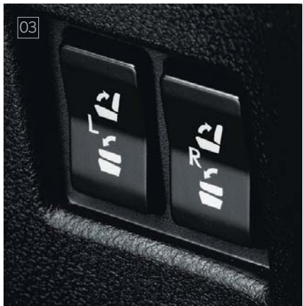
02 / Power Back Door *1 Convenient controls for the power door are set in the instrument panel and Electronic Key, as well as a closing switch in the bottom of the door. 03 / Power Rear Seats *2 Enhancing versatility and convenience, the rear seats can be reclined, folded flat or upright at the touch of a button integrated into each seat, in the luggage space, and the driver's side instrument panel.
